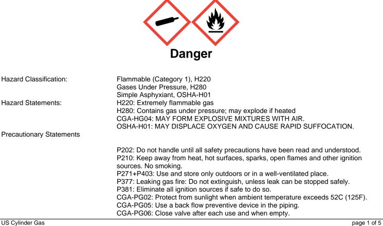
CGA-PG10+CGA-PG20: Use only with equipment of compatible materials of construction and rated for cylinder pressure. CGA-PG12: Do not open valve until connected to equipment prepared for use. CGA-PG27: Read and follow the Safety Data Sheet (SDS) before use.
